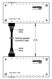
The following draft shows an assembled s88 connection cable shown from the left side.
