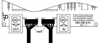
Attach the second pin-socket of the bus-cable directly to the command station or to the interface respectively to an other feedback module within the feedback line.
