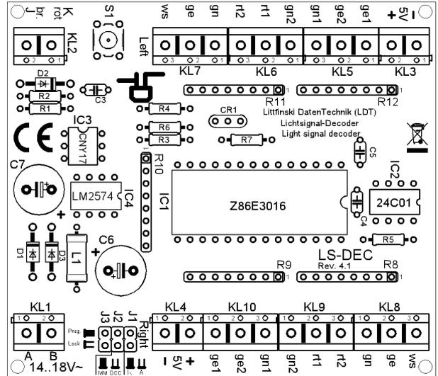
**Lenz-Digital systems** are using the letters '**J**' and '**K**'. In case you assemble the decoder to an **Arnold-Digital (old)- or Märklin-Digital=** system, you have to connect '**black**' to '**K**' and '**red**' to '**J**'.
