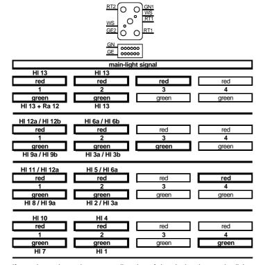
If you do not know the correct allocation of the single wires to the light emitting diodes you can **test** the function by connecting the wires to **clamp RT1**. This output is **active** because the decoder switches **all signals to red after switching on**.
