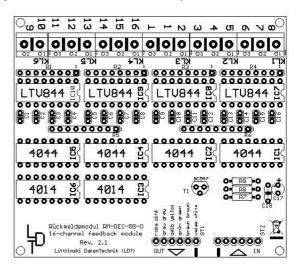
The feedback module **RM-DEC-88-O** is suitable for decentralized installation below the model railway layout. There are 4 bores on the pc-board for quick and easy installation. A suitable installation kit consisting of four distance spacers and four wood-screws is available under the order code MON-SET. An exact matching case for the feedback module can be ordered under coder LDT-01.
