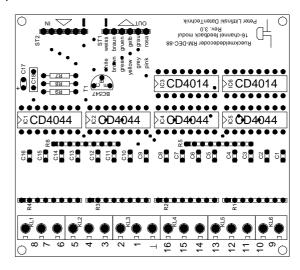
The feedback module **RM-DEC-88** is suitable for decentralized installation below the model railway layout. There are 4 bores on the pc-board for quick and easy installation. A suitable installation kit consisting of four distance spacers and four wood-screws is available under the order code MON-SET. An exact matching case for the feedback module can be ordered under coder LDT-01.
