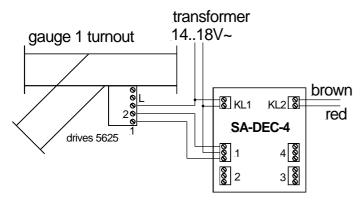
Feed the **SA-DEC-4** via **KL1** witch **AC** from the **model railway transformer**. Further connect one cable of the transformer with clamp **'L'** at the turnout drive. Connect the second cable of the transformer with the clamp marked with **'COM'** on the respective decoder output.
