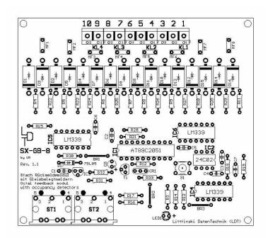
The **SX-GB-8** contains an **automatic overload fuse** on each of the 8 outputs to protect the connected central unit or the boosters by possible current overload or short circuit. Is a short circuit eliminated the respective output will start up again to supply digital-current to the monitored track section after some seconds.
