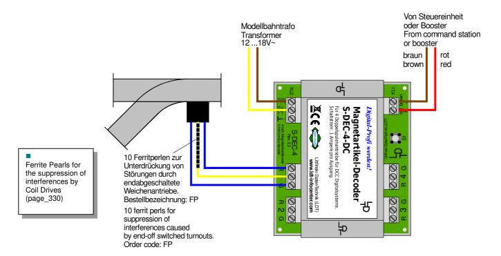
The ferrite pearls are available by LDT under the order code "FP". The connections and the operation of the turnouts as well as the programming the decoder will not be influenced.
