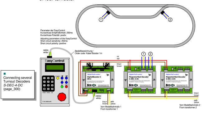
It is recommended to install a separate second main ring conductor for the digital current to the turnout- and switch decoders (**red** / **brown**) and a third main ring conductor for the voltage supply (**yellow** / **brown**).
