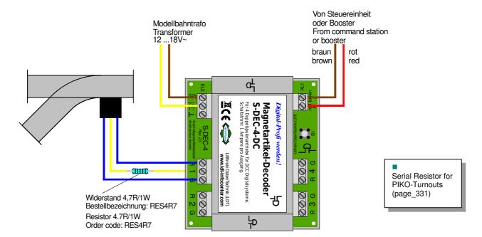
The resistor is available as accessory by LDT under the order code "RES4R7". There will be no change within the connections or the operation of the turnouts as well as on the programming of the decoder. For the suppression of interferences by those end-off switched turnouts is it recommended to apply the ferrite pearls as well on the common connection (yellow) of the turnouts ⇒ "Suppression of interferences" (Page 6).
