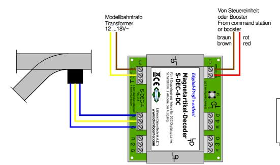
Connection of the Turnout-Decoder S-DEC-4-DC (page\_329)
