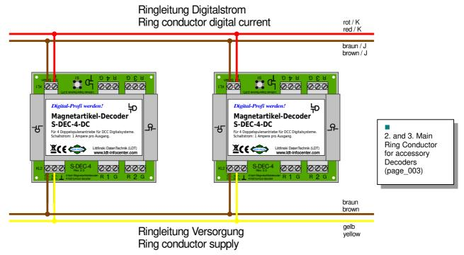
There are as well some recommendations for the wire cross-section dimension to be used for the two main ring conductor wires. As there will be a low current flow only, the wire dimension can be a little smaller.
