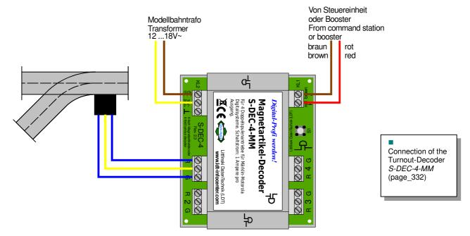
Power supply (yellow / brown cables at the above sample) will be required for the module itself and for the switching of the coil drives. The decoder module requires a spacing current flow of about 0.1 Ampere. Each output can cover a maximum switching current load of up to 1 Ampere.
