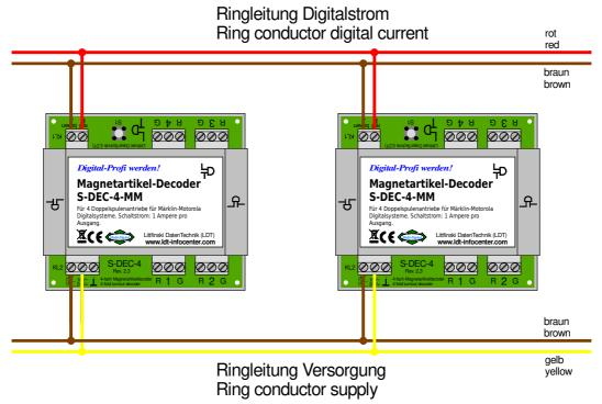
There are as well some recommendations for the wire cross-section dimension of the two main ring conductor wires. As there will be a low current flow only the wire dimension can be a little smaller.
