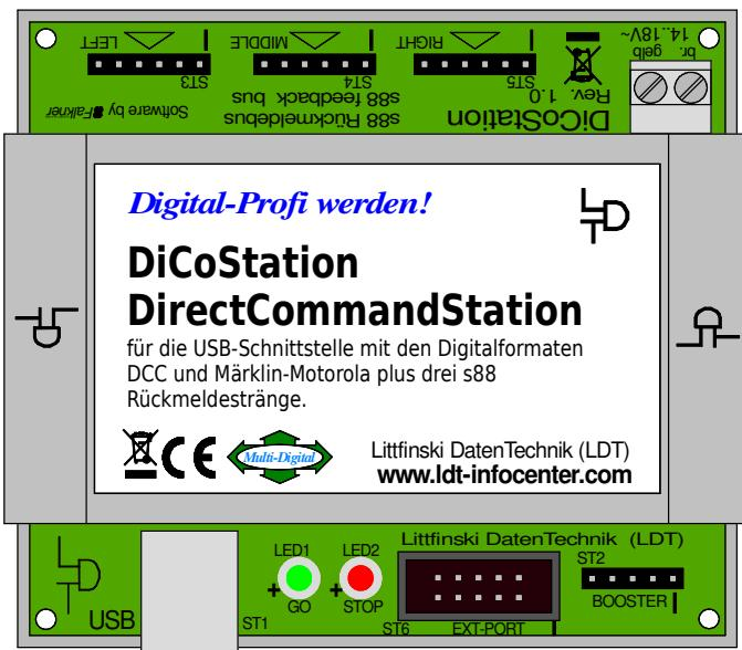
The DiCoStation is a digital command station for monitoring and control of your digital model railway layout with a PC-Software (e.g. Railware, TrainController, WinDigipet).
