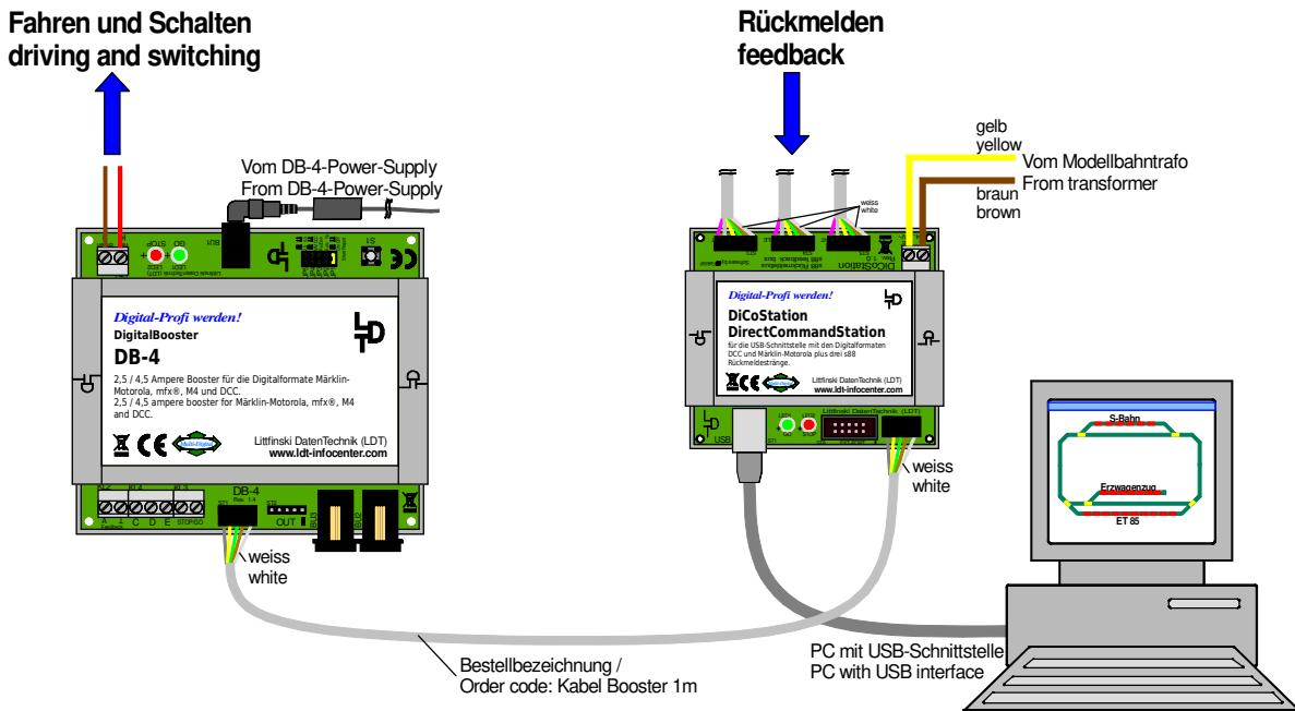
The DiCoStation will be connected to the DigitalBooster DB-4 via the 5 poles booster bus and get the AC power supply from a model railway transformer (14 to 18V).
