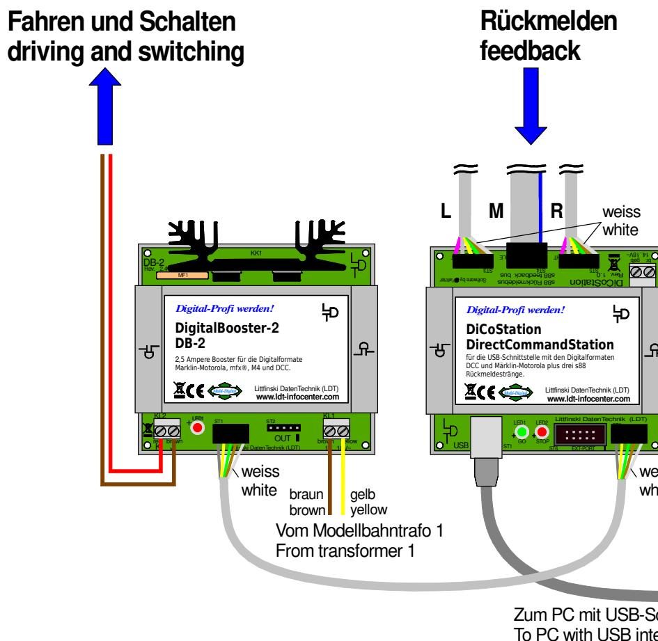
**s88-standard bus connections** are correct plugged to the three 6-poles pin bars of the **DiCoStation**. On the pin bar of the middle bus line has been a flat ribbon bus cable attached.
