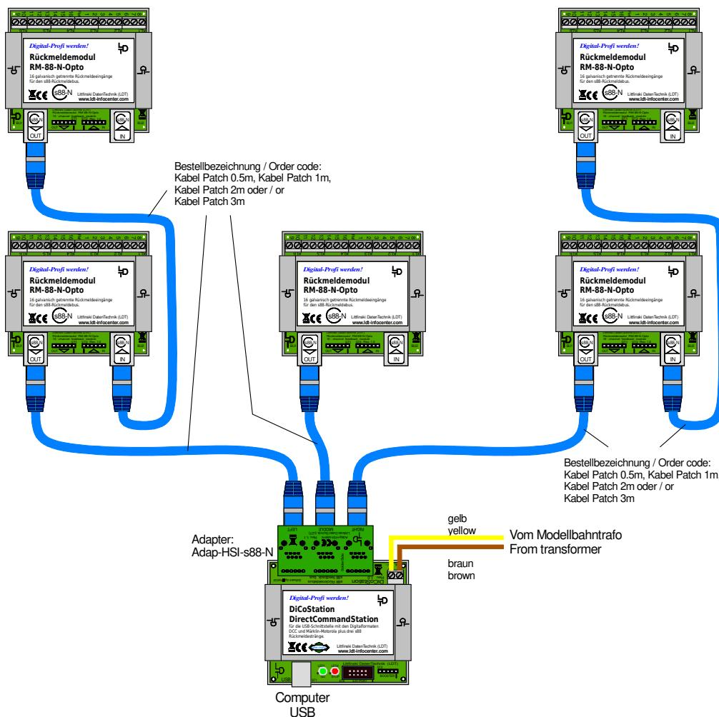
If the DiCoStation will be extended by the adapter Adap-HSI-s88-N is it possible to use screened patch cables as s88-bus cables to the first feedback module.
