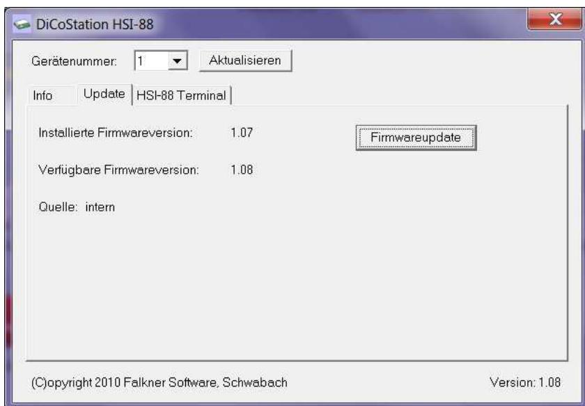
**Important Information:** The **device number** should **never be changed**. Otherwise the model railway software will not **recognize** the **HSI-88-USB** any more. The device number will be important as soon as you use more than one **HSI-88-USB** or **additionally a DiCoStation for driving and switching**. The first **HSI-88-USB** will get automatically always the **device number 1**.
