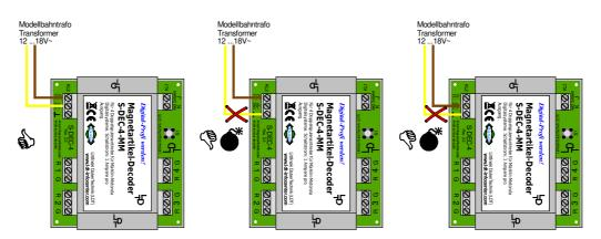
Correct connection of the external supply voltage (page\_509)
