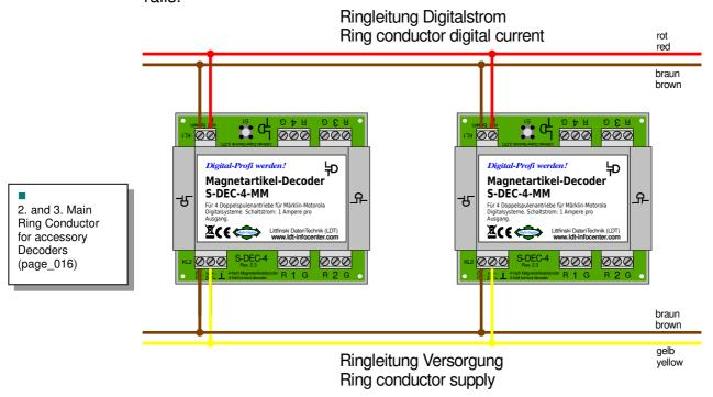
There are as well some recommendations for the wire cross-section dimension of the two main ring conductor wires. As there will be a low current flow only the wire dimension can be a little smaller.
