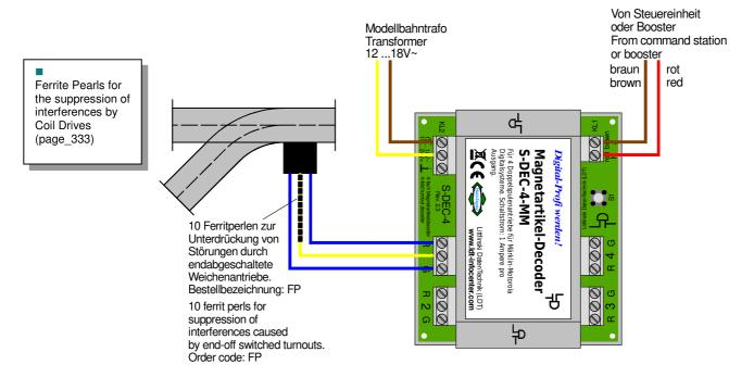
The ferrite pearls are available by LDT under the order code "FP". The connections and the operation of the turnouts as well as the programming the decoder will not be influenced.
