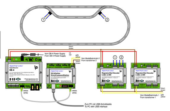
It is recommended to install a separate second main ring conductor for the digital current to the turnout- and switch decoders (red / brown) and a third main ring conductor for the voltage supply (yellow / brown).
