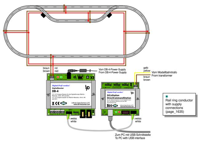
Each plugged rail connection will contain an electrical resistance. This resistance will be enlarged by corroded contacts etc.
